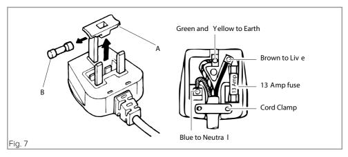
The mains lead of this appliance has been fitted with a BS 1363A 13 Amp fused plug. To change a fuse in this type of plug, follow the steps below:
