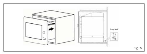
• Open the appliance door and fix the appliance in position using the supplied screw in the installation hole.
