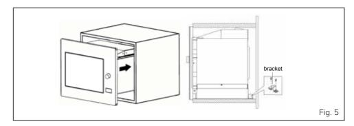
• Open the appliance door and fix the appliance in position using the supplied screw in the installation hole.
