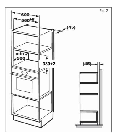
• Use the supplied template to mark out the 2 holes for the rear fixing bracket on the centre line of the tall cabinet.
