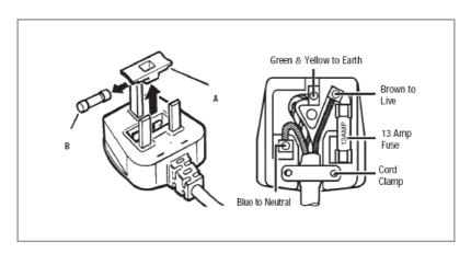
The mains lead of this appliance has been fitted with a BS 1363A 13 amp fused plug. To change a fuse in this type of plug, follow the steps below:
