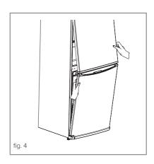
3. Remove the kick plate by pulling forwards. Remove the lower hinge fixing screws and the lower hinge. Unscrew the lower hinge pin from position 1 in fig. 5, rotate the lower hinge 90° and then screw the hinge pin into position 2. Relocate the lower hinge into position on the left hand side using the lower hinge fixing screws.
