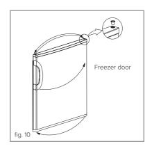
8. Rotate the central hinge 180°.
