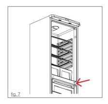
5. Unscrew the upper hinge pin and screw it into position of the left hand side (fig. 8).
