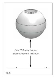
Where the extractor is to be installed above a non-CDA hob, the instructions supplied with the hob may dictate that the height required above the hob is greater than 650mm.
