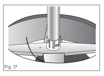
Insert the top tube into the ceiling bracket and secure it with two supplied through-bolts and nuts (Fig 18).
