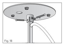
12. Pass the end of the safety cable up through its hole in the top of the sphere (marked "A" in Fig. 19). Then fit the cable clamp to it.
