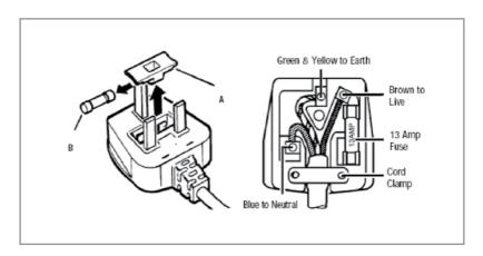
The mains lead of this appliance has been fitted with a BS 1363A 13 Amp fused plug. To change a fuse in this type of plug, follow the steps below:
