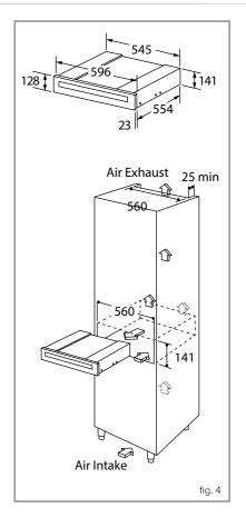
The top of the unit should be open to allow air to escape and a free air intake should be provided in the housing unit to allow a natural flow of cooling air inside the unit. The dimensions of the air intake are recommended as 500mm x 25mm (or 1250cm²).
