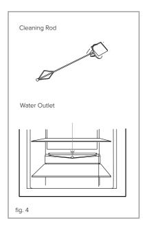
The water drain hole at the back of the fridge compartment and the evaporating tray should be cleaned periodically to prevent the defrosted water from collecting inside the fridge compartment. The drain plug can be used to clean the drain hole.
