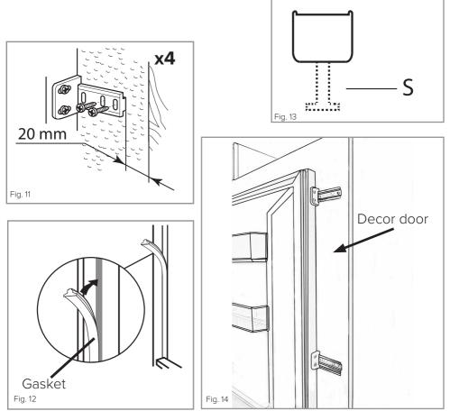
Important: After completing the installation, check that the appliance is secured within the unit and that the door(s) close and open properly. If there is no resistance from the door seals when opening the doors, then it is probable that the appliance and/or decor doors are not fitted properly.
