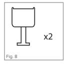
Ensure that the lips of the spacers are level with the lip of the cabinet base.
