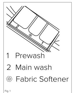
The detergent dispenser is designed to allow the use of liquid detergents rather than adding them to the drum. You should only insert liquid detergent into the main wash detergent compartment and ensure that concentrated liquid detergent is diluted with an equal quantity of water before use.
